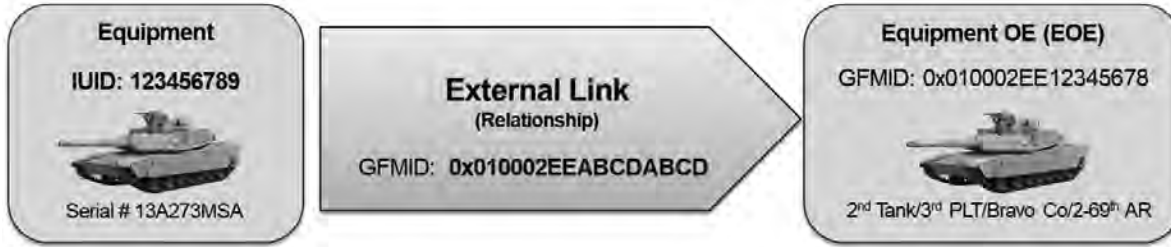
Figure 22-15. Linking the Crewed Equipment (Tank IUID) to the EOE (GF MID) that is Associated with the Crew
